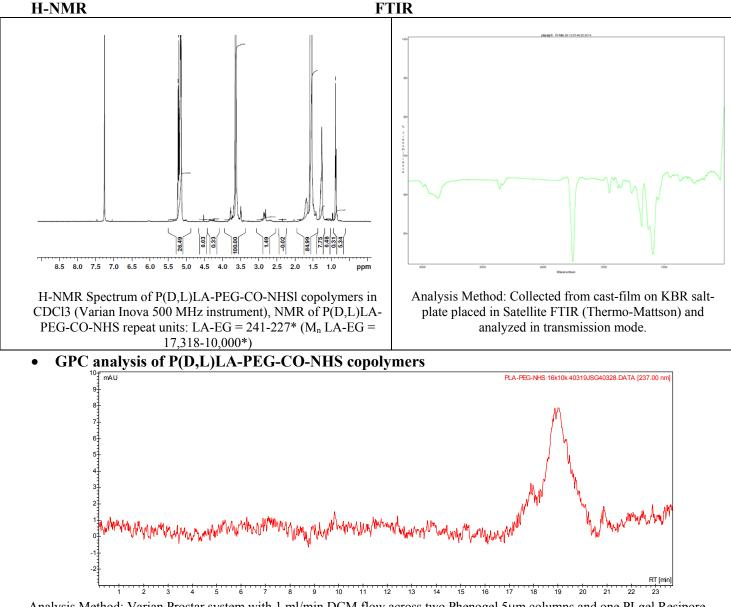
Analysis Method: Varian Prostar system with 1 ml/min DCM flow across two Phenogel 5µm columns and one PLgel Resipore column (Agilent). Detection via UV/Vis, calibrated against polystyrene standards
